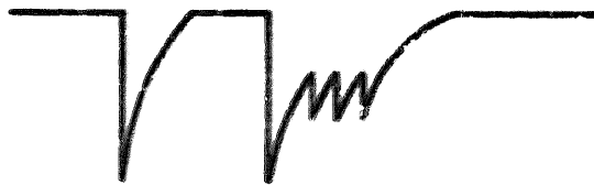
Figure 5-3. Isolated Track Pulse at TP7.
